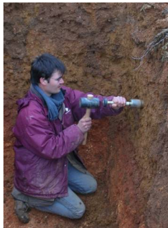
Photo 3. Measuring the bulk density of the soil
